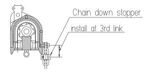
Checking of the install position for the attachment of lifting and lowering limiter.
